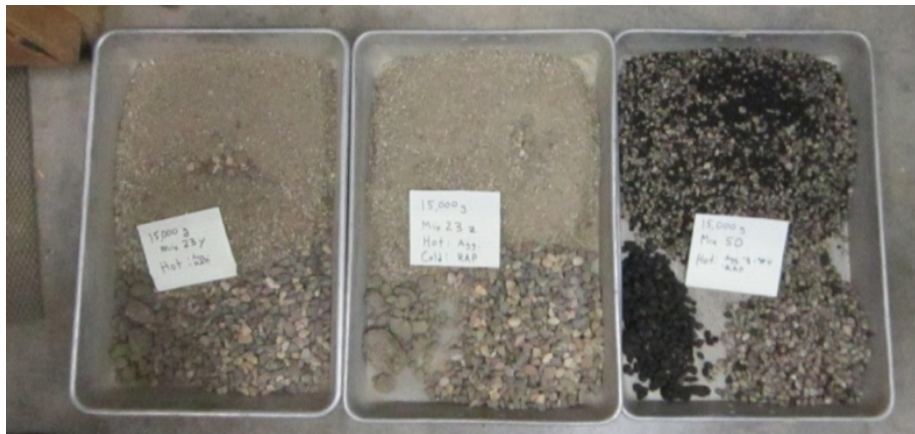
Figure 10: Examples of 15,000 gram Lab Activation Trials at 23 and 50% RAP
